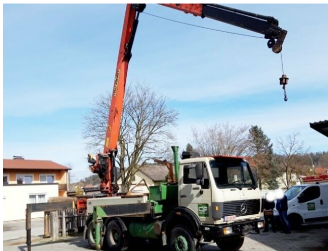
Mercedes-Benz 2635 6x4 2635 6x4, V8, Heckkran Palfinger PK 28000, Funk, 28,5m-280kg
