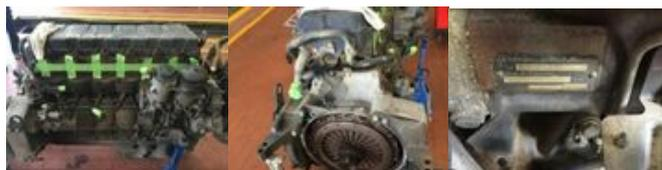
**MAN Motor D2066LF31 Motor D2066LF31, 6-Zylinder**
