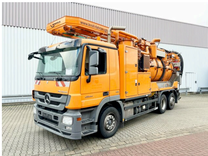
Mercedes-Benz Actros 2544 L 6x2 Actros 2544 L 6x2, Lenkachse, Kroll Saug-/Spülwagen ca. 12m 3 , Funk
