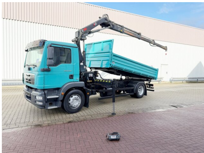
MAN TGM 18.290 4x2 LL TGM 18.290 4x2 LL, EEV, Kran Hiab XS 111 ES-3 HiDuo, Funk
