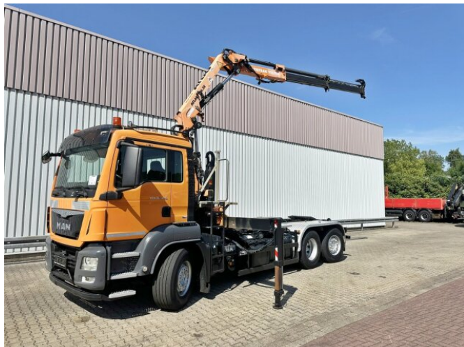
MAN TGS 28.440 6x2-4 BL TGS 28.440 6x2-4 BL, Kran Atlas 126.3E-A2L, Funk, Lenk-/Liftachse
