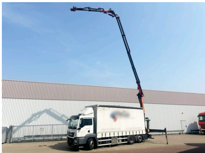
MAN TGS 26.400 6x2-4 LL TGS 26.400 6x2-4 LL, Heckkran Palfinger PK23002-C + Jib PJ060A, Funk, Lenk-/Lift, Edscha
